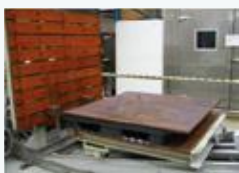
Pallet underwent Collapse Resistance Test
